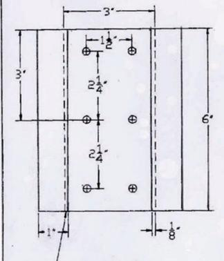
Legs are welded & inset from edge of leg bracket.
